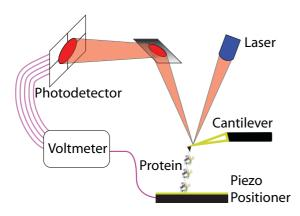
FIG. 1. (Color online) Schematic representation of a typical AFM setup for protein measurements. The deflection of the cantilever is measured as a differential voltage on the quadrant photodetector. In order to achieve a force measurement one must convert the voltage measured on the photodetector into a displacement of the tip and then measure the spring constant of the cantilever (typically done using the thermal tune method [14]).
